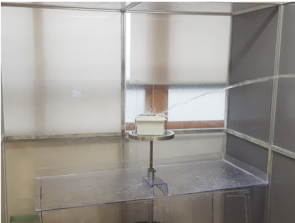
[Photo – waterproof test]
