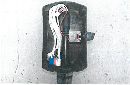
Figure 18) Photo of the specimen after the test (IP6X, #1)
