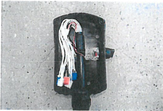
Figure 20) Photo of the specimen after the test (IPX5, #1)
