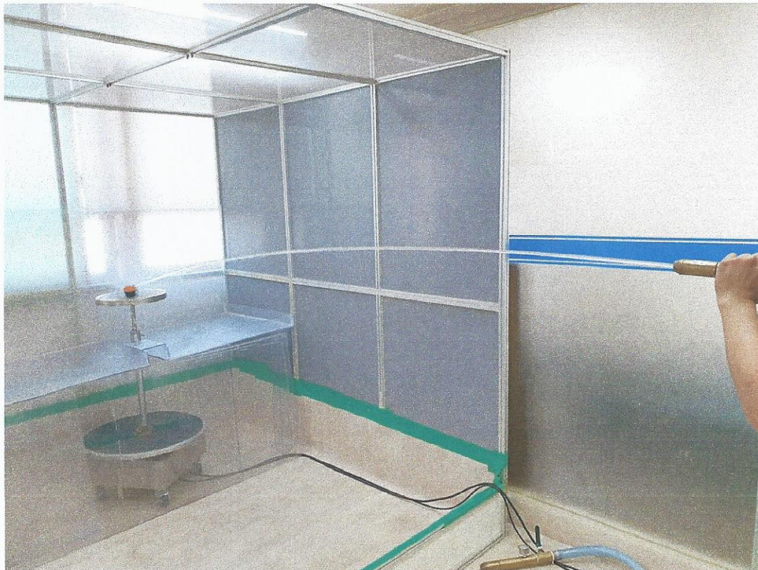
[Photo 5 - during the waterproof test]
